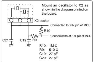
Figure 4 Connection diagram of X2 socket
